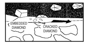
Eventually the diamond completely breaks up and it's fragments are swept away with the material that it is grinding.
