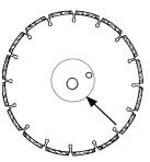
CAUSE: Blade collars are not properly tightened or are worn out. REMEDY: Check tightness and replace colif necessary. lars
