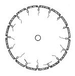
CAUSE: Blade is too hard for material being cut.
