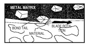
Diamond blades don't cut, they grind ! The exposed diamond crystals do the grinding work. The metal matrix or bond holds the diamonds in place. Trailing behind each exposed diamond is a "bond tail" which helps to support the diamond. As the blade rotates through the material the exposed surface diamonds grind the material being cut into a fine powder
