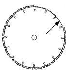
CAUSE: On stone or masonry blades the material may not have been held firmly which allowed the blade to twist or jam. REMEDY: Material must be held firmly.
