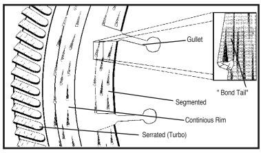
A diamond blade is a circular steel disc with a diamond bearing edge. The edge or rim can have either a segmented, continuous or serrated rim configuration.
